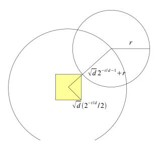
Figure 4: If the query point falls more than  $\sqrt{d}2^{-t/d-1} + r$  away from the center of a box it cannot be 'hit'.
