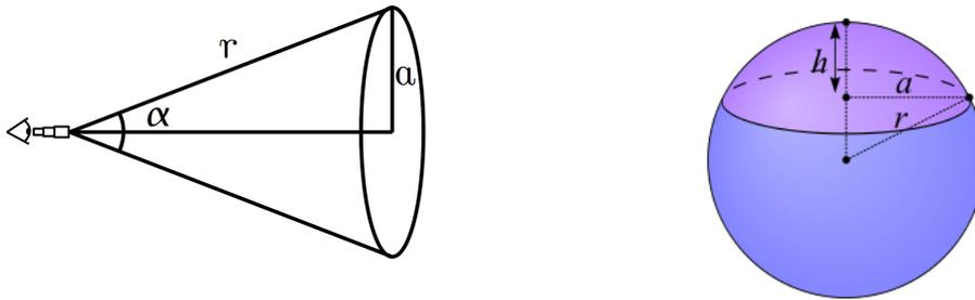
Figure 1: On the left: an illustration of the visual angle  $\alpha$  of a telescope ( $\sin(\alpha/2) = a/r$ ). On the right: a spherical cap of base  $a$  and height  $h$  on a sphere of radius  $r$ . The area of the spherical cap is  $2\pi rh$ . The surface area of the entire sphere is  $4\pi r^2$ .
